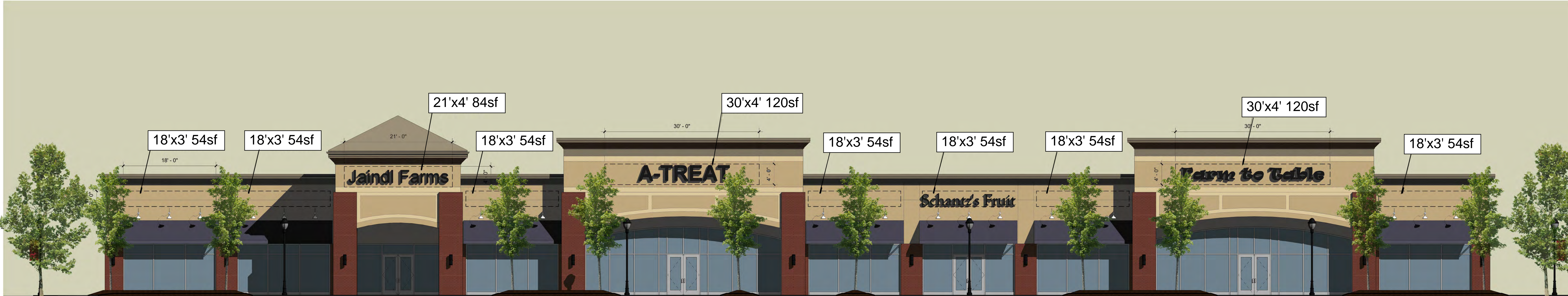
1 South 1/8" = 1'-0" Proposed Building Elevation Area = 7,088sf, 10% Signage Area = 708sf, Total Proposed Signage Area = 702sf
