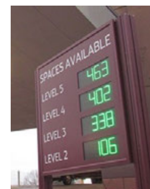
Wayfinding and signage showing parking availability reduces traffic and driver frustration
